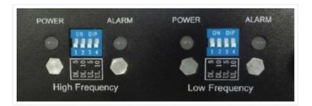
Put ON a pair of switches for a total of 15dB reduction in gain. (DL1 & UL1 - Alarm Low) - For 800MHz or 900 MHz Band (DL2 & UL2 - Alarm High) - For 1700, 1800, 1900 & 2100 MHz Band
