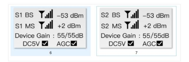
**LINE 1.** BS shows the level of outdoor incoming signal for the corresponding frequency band. Make sure it is as low as possible.
