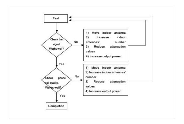
For maximum precision in signal level testing, switch your cell phone into Field Test Mode and see dB parameter. The closer dB signal level to 0, the better cell phone reception you'll get.
