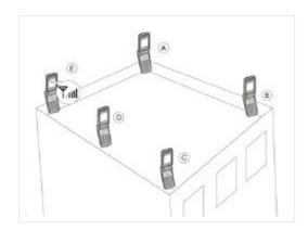
The repeater's main function is to improve weak RF signals in an area. The formula is: Input power + Gain= Output power. The signal strength from an outdoor antenna directly affects the efficiency of the indoor coverage. It is very important to choose the correct outdoor antenna location in order to get the best signal.
