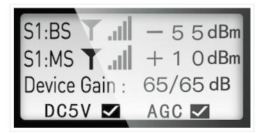
**LINE 1.** BS shows the level of outdoor incoming signal for the corresponding frequency band. Make sure it is as low as possible.
