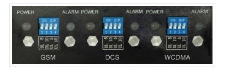
Put ON a pair of switches for a total of 15dB reduction in gain. You can reduces anyone system in the products.
