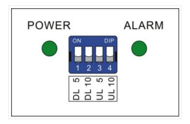
DIP switch uplink attenuation setting:
