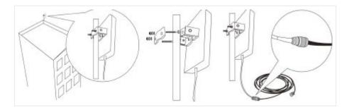
Installation of Yagi wide band antenna as an outdoor antenna
