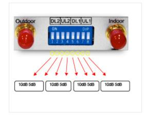
Put ON a pair of switches for a total of 15dB reduction in gain. (DL1 & UL1 – Alarm Low) – For 800MHz or 900 MHz Band (DL2 & UL2 – Alarm High) – For 1700, 1800, 1900 & 2100 MHz Band
