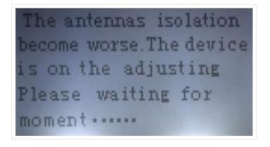
If the device detects self-oscillation between the antennas and says that the system is being adjusted, it means that the system has detected the problem of bad isolation between the antennas and AGC is adjusting the system gain automatically to make the device work correctly. No actions are required from you.
