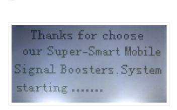
Introduction screen. The introductory page is displayed at the screen for 10 sec during the system checkup.
