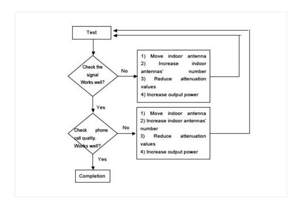
For maximum precision in signal level testing, switch your cell phone into Field Test Mode and see dB parameter. The closer dB signal level to 0, the better cell phone reception you'll get.
