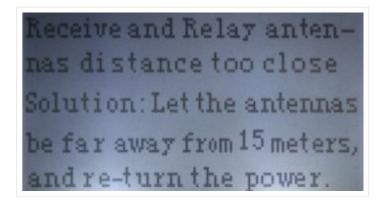
If the device detects that the outdoor antenna is too close to the indoor, change the position of either or both antennas to avoid self-oscillation. Mount them at least 15m one from another.
