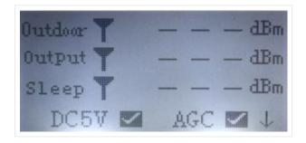
When the device completes the internal self test, it shows the standby screen. If the arrow down is displayed at the bottom right corner, the device has detected signal reception problems. In this case press Page Down button to see possible solutions. Resolve the issue basing on the recommendations. (see possible troubles and solutions below in Questions & Solutions paragraph)
