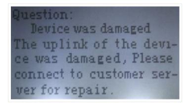
If the system shows "Device was damaged" note, it means that the uplink/downlink was damaged. Contact customer service for repair.
