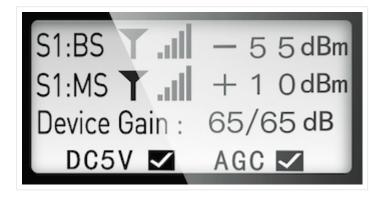
**LINE 1.** BS shows the level of outdoor incoming signal for the corresponding frequency band. Make sure it is as low as possible.
