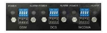
Put ON a pair of switches for a total of 15dB reduction in gain. You can reduces anyone system in the products.
