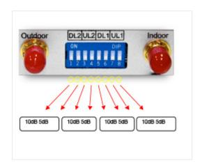
Put ON a pair of switches for a total of 15dB reduction in gain. (DL1 & UL1 - Alarm Low) - For 800MHz or 900 MHz Band (DL2 & UL2 - Alarm High) - For 1700, 1800, 1900 & 2100 MHz Band
