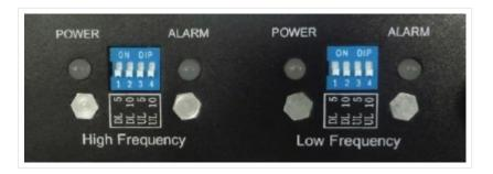
Put ON a pair of switches for a total of 15dB reduction in gain. (DL1 & UL1 - Alarm Low) - For 800MHz or 900 MHz Band (DL2 & UL2 - Alarm High) - For 1700, 1800, 1900 & 2100 MHz Band
