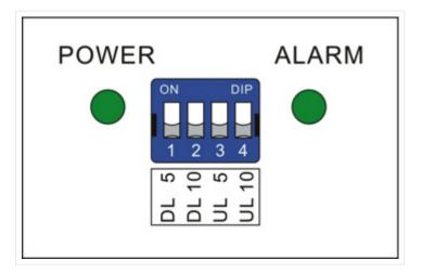
DIP switch uplink attenuation setting:
