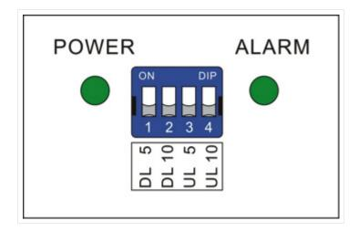
DIP switch uplink attenuation setting:
